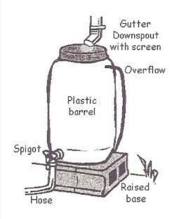
5. Using an overflow spigot or hose, send the overflow water away from the building. The overflow water can be used to water rain gardens, washcars, or can go directly to a city drain.
